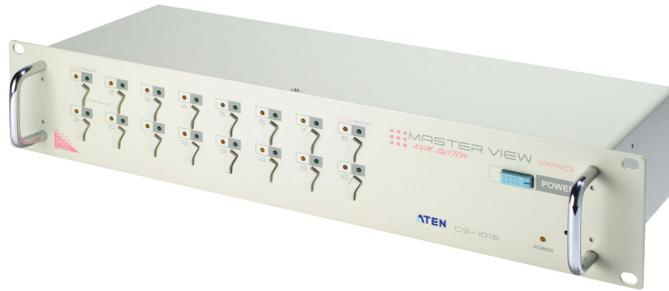
CS1016 KVM Switch is designed according to the needs of server rooms of larger scale. It uses the DB-25 interface to integrate relevant signals, reduce cable derangements, and enhances signal quality and operation efficiency. CS1016 supports OSD (On Screen Display) menu function to facilitate operators to switch between computers. It also supports microphone and amplifier functions.
