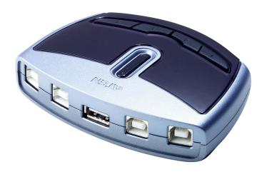
US421 allows 4 computers to share the same USB peripheral under the foundation of one-at-a-time. Users can switch the computer controlling the peripheral from the simple hotkeys or buttons on the front panel or the control software on Windows. It is ideal for SOHO environments.
