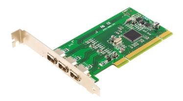
IC1394 is a hub with 3 built-in IEEE 1394 ports for expanding computer peripherals.
