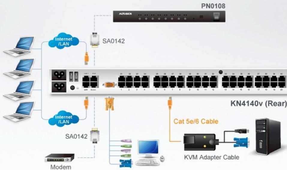
4 remote buses – 4 remote consoles can simultaneously access separate ports – up to 32 users can share the remote buses.
