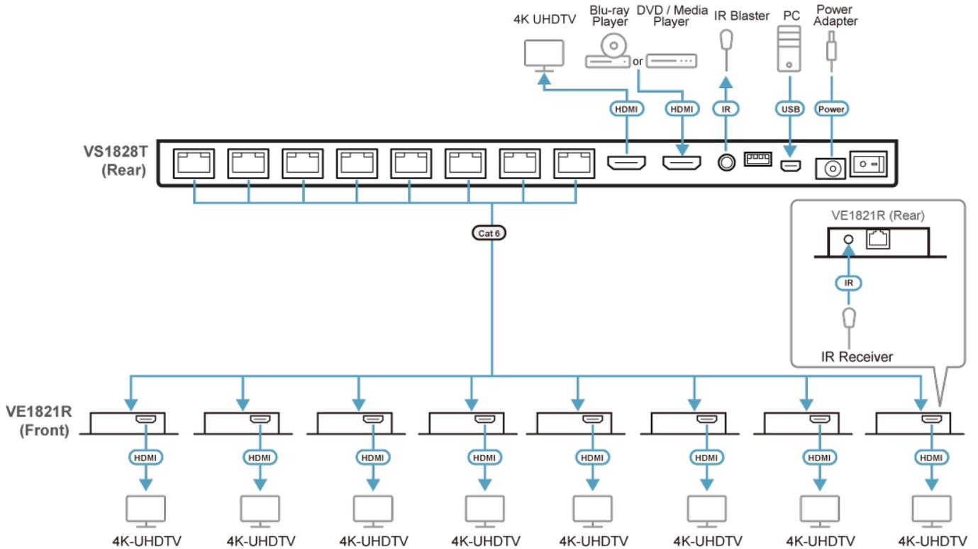
Note: Only connect VS1828T with VE1821R. Connecting VS1828T with other receiver models or third-party receivers may cause physical damage to the receiver.
