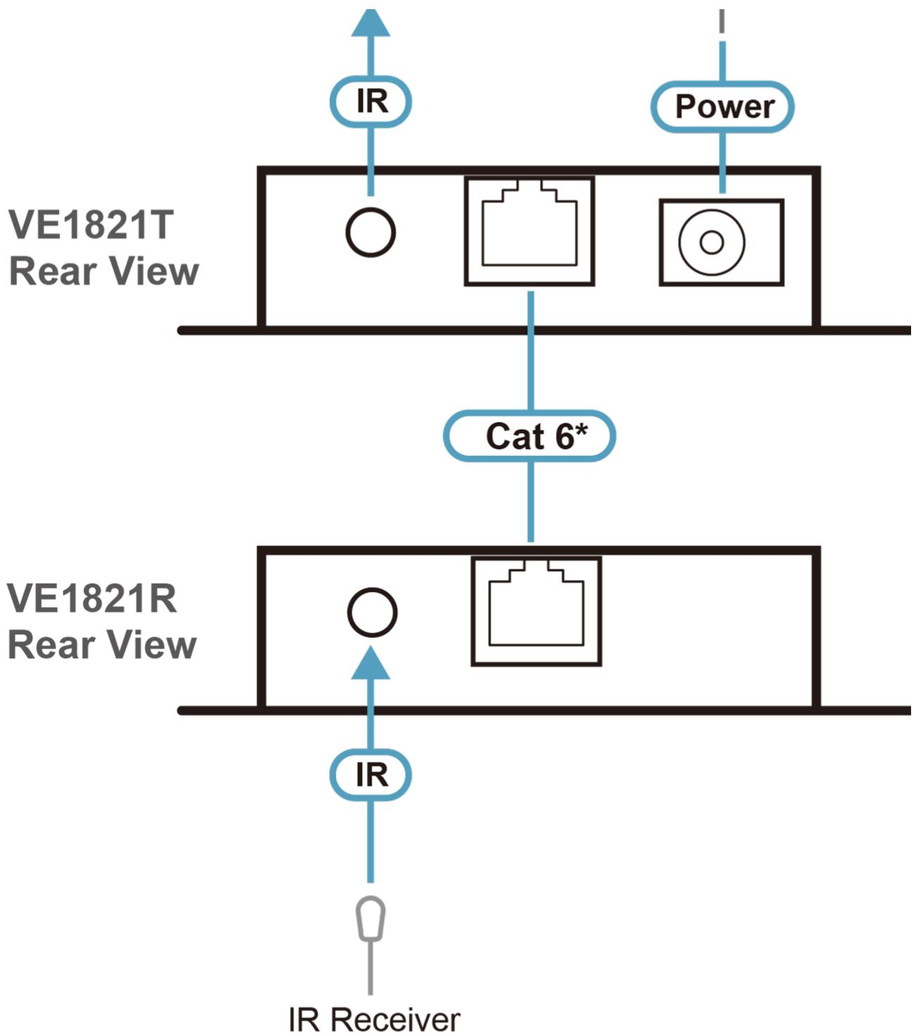
Note: Make sure to only connect VE1821T with VE1821R using models or third-party receivers may cause physical damage
