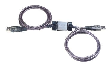
The UN201 provides a quick and easy solution for host-to host peer networking communication. Users can now network two or more USB computers through standard plug-and play technnology without adding network cards. Share files and resources(printers,scanners,modems,CD-ROM drives,etc).
