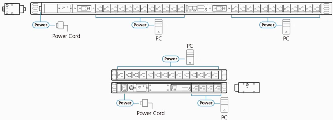
Note: As there are many Basic Metered PDUs, PE1324S (top) and PE1118S (bottom) are the respective 0U and 1U examples used here.
