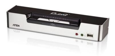
The CS1642 USB 2.0 DVI Dual View KVMP™ Switch charts a revolutionary new direction in KVM (Keyboard, Video, Mouse) switch functionality by combining a 2-port KVM switch with a 2-port USB 2.0 hub at the same time as providing dual-screen support for two DVI displays, making it ideal for graphic designers, banking and finance consultants, medical applications, and gamers.
