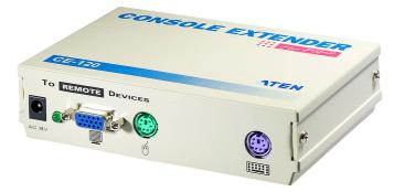
CE120 KVM Verlenger is a console verlenger with built-in PS/2. It allows remote users to connect and access to the server devices via the console. Users will only need to install it by connecting some cables, without using additional tools or software.
