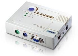
CE220 KVM Verlenger is a console verlenger with built-in PS/2. It allows remote users to connect and access to the server devices via the console.
