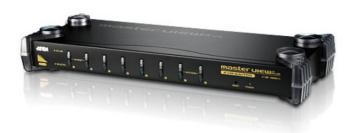
KVM Switch can control 8 computers and connect computers in 3 tiers via cascade. With 73 sets of CS88A, users can manage up to 512 computers from the console.
