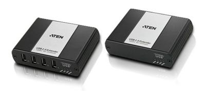
The UEH4002 incorporates patented ExtremeUSB ® technology that enables users to extend beyond the standard 5 m cable limit for USB peripheral devices. Up to 14 USB devices can be connected to the Remote unit up to 100 meters from the computer.
