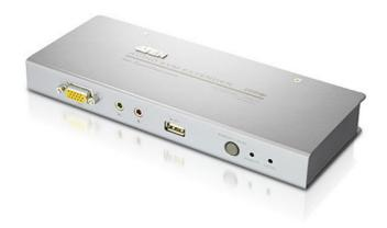
The CE800 allows access to your KVM installation through a local console, or a remote console placed up to a distance of 250m(825ft) away. Both the local and remote unites support USB consoles(monitor, keyboard, and mouse), with the addition of a USB peripheral port on each unit. This port provides file swapping from mass storage devices and includes file sharing security features.
