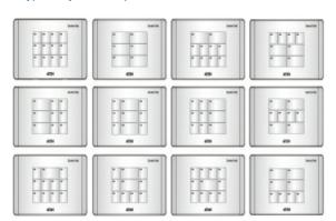
Custom button placement on the Control Pad can be set in 125 different combinations of 6 to 12 buttons. The example above shows the 12 most commonly used.
