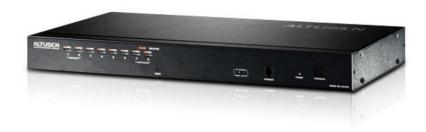
The KH1508 KVM Switches are control units that allow access to multiple computers from a single KVM (keyboard, monitor, and mouse) console. The KH1508 features RJ-45 connectors and Cat 5e/6 cable to link to the computers. Combined with Auto Signal Compensation (ASC) signals can travel up to 40 meters and still maintain high video resolution.
