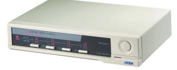
CS124A is a KVM switch with built-in PS/2. It can control 4 servers via a single console and allows users to switch between computers via the buttons on the upper part of the switch or the hotkey configuration on the console keyboard. Moreover, it can control up to 64 computers via cascade.
