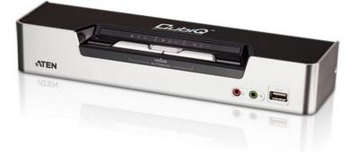
The CS1642 USB 2.0 DVI Dual View KVMP<sup>™</sup> Switch charts a revolutionary new direction in KVM (Keyboard, Video, Mouse) switch functionality by combining a 2-port KVM switch with a 2-port USB 2.0 hub at the same time as providing dual-screen support for two DVI displays, making it ideal for graphic designers, banking and finance consultants, medical applications, and gamers.
