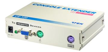
CE120 KVM Extender is a console extender with built-in PS/2. It allows remote users to connect and access to the server devices via the console. Users will only need to install it by connecting some cables, without using additional tools or software.
