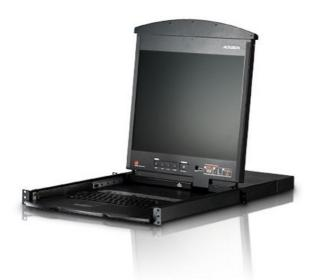
ALTUSEN KL1508 LCD KVM Switch features independently retractable, dual slide 17" or 19" LCD monitor and keyboard with built-in touchpad. A single KL1508 can control up to 8 computers. For increased reliability and efficiency, RJ-45 connectors and Cat 5e/6 cable are used to link to the computers. Utilizing KVM Adapter Cables for the final linkup, the KL1508 permits any combination of PCs, Macs, Sun computers, and serial devices to coexist on the installation.
