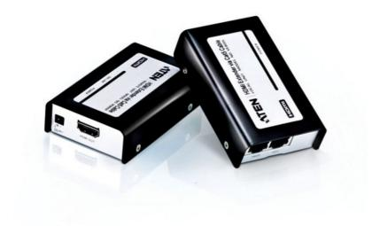
The VE800 HDMI Extender extends your HDMI display up to 60 m away from your HDMI source using two Cat 5e cables. It is equipped with HDMI (high definition multimedia interface) connectors and is capable of supporting DVI-D (Single-Link) equipment when used with a HDMI-to-DVI adapter, providing greater flexibility and installation options when integrating several home theater components.
