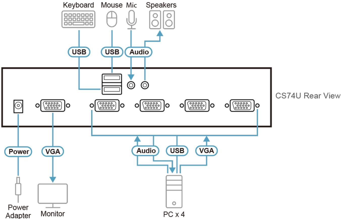
**!** The CS74U is bus-powered, which draws power from the connected PCs. To provide enhanced power via the built-in power jack, it is required that you use a compatible ATEN power adapter. Please contact your ATEN dealer or Technical Support for detailed information.
