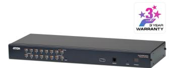
The KH1516A KVM switches are control units that allow IT administrators to access and control multiple computers from a single PS/2 or USB KVM console (keyboard, monitor, and mouse). Operators can take control of up to 16 computers. By daisy chaining up to 31 additional switches, as many as 512 computers can be controlled from the original KVM console.
