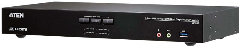
The ATEN CS1842 Dual Display KVMP™ Switch presents a valuable solution for desktop workstation with instant and effortless access to two HDMI interface computers from a single USB keyboard, mouse and two HDMI monitors; to meet users' needs, the CS1842 is compliant with HDMI 2.0 standard and supports superior video quality up to 4K DCI (4096 x 2160 @ 60Hz), offering the most stunning and vivid visuals.
