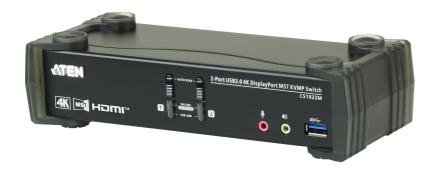
Incorporating the latest Multi-Stream Transport (MST) technology, the CS1922M 2-Port USB 3.0 4K DisplayPort MST KVMP<sup>TM</sup> Switch is the world's first DisplayPort KVM switch with a built-in MST hub. The CS1922M enables users to adopt two console displays from a single DisplayPort 1.2 video source, providing an extended desktop mode and splitter mode at resolutions up to 4K for multitasking across two displays while reducing bulky cable connections.
