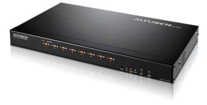
The KN9108 allows two administrators - one logged in at a local console; the other logged in remotely from any IP connected web browser and up to 32 users to securely monitor, manage, troubleshoot or run applications from up to 8 connected devices respectively.
