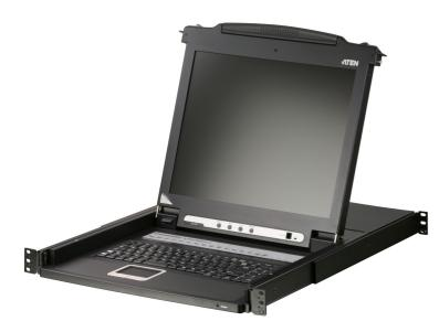
The CL1016 LCD KVM Switch series are control units that allow access to multiple computers from a single keyboard, video, and mouse (KVM), console. A single CL1016 can control up to 16 computers. As many as 15 additional KVM switches can be daisy-chained to the CL1008, so that up to 256 computers can all be controlled from a single KVM console.
