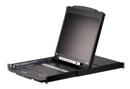
The CL5808 Slideaway™ Dual Rail LCD KVM Switch is a control unit that allows access to multiple computers from two PS/2 or USB KVM consoles. An extra console port is provided on the rear panel to manage the LCD KVM switch from an optional external consoles.
