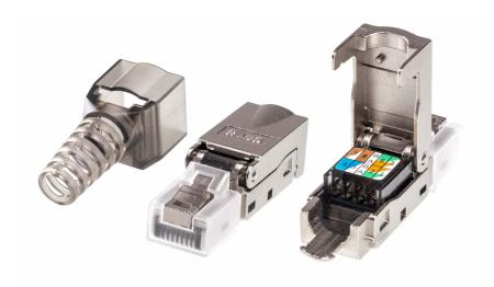
The ATEN 2A-245G Cat 6A RJ-45 metal-shielded connector offers excellent electromagnetic interference protection, supports over 10G data transfer, and meets FCC Part 68 standards. Its reinstallable and die-cast RJ-45 design ensures stable transmission and durability with over 750 mating cycles. It's compatible with PoE / PoH and works well with various cable types, especially 2L-29330 Cat 6A cables.
