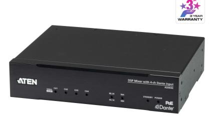
The AD004E converts Dante inputs into 4-channel analog line outputs, integrating analog and digital audio devices into one single system through Dante AoIP media networking technology. It supports 24 bit and offers sampling rate options of 44.1k, 48k, 88.2k, and 96 kHz to meet different environment needs.
