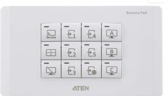
The VPK312 is a 12-key, network-based remote pad designed for use with ATEN Presentation Switches. It offers an intuitive interface for function control of the connected Presentation Switch from a standard 2-gang EU wallmounted keypad. Created with flexibility in mind, the functions and layout of the keys can be easily customized via an intuitive web GUI to meet different application requirements
