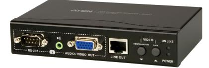
The VB552 VGA Over Cat 5 Repeater +Audio is an audio/video signal extension device which is compatible with ATEN Cat 5 Audio/Video splitters. The VB552 extends the audio/video transmission range an extra 150m over Cat 5e (or higher) cables. The use of an additional repeater means the audio/video signals can be transmitted over even longer distances, up to 450m.
