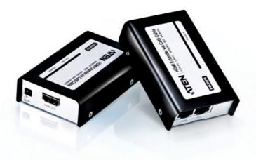
The VE800 HDMI Extender extends your HDMI display up to 60 m away from your HDMI source using two Cat 5e cables. It is equipped with HDMI (high definition multimedia interface) connectors and is capable of supporting DVI-D (Single-Link) equipment when used with a HDMI-to-DVI adapter, providing greater flexibility and installation options when integrating several home theater components.
