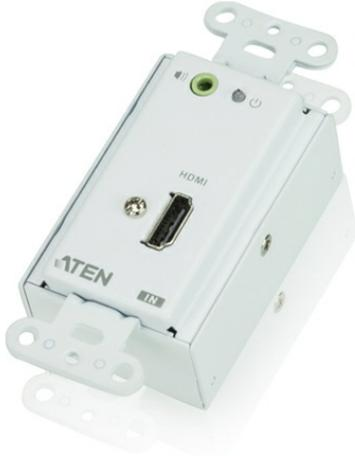
The VE806T HDMI Over Cat 5 Transmitter Wall Plate connects to a [VE806R](#) to extend signals up to 60m from the source using Cat 5e cables. It supports popular wide screen formats and ensures excellent video quality over long distance transmissions. The [VE806](#) combination can further extend the distance or multiply sources/displays.
