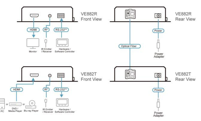
\* The IR bypass channel is bi-directional. The IR transmitter and IR receiver can be plugged either into the VE882T or VE882R unit depending on the device you want to control remotely.
