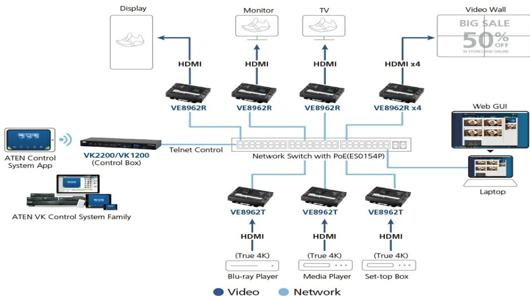
Note: VE8962 supports PoE and can be installed in combination with PoE network switches to reduce power cabling and additional power outlets. Before choosing the Network switch and installation, please refer to the Implementation Guide.
