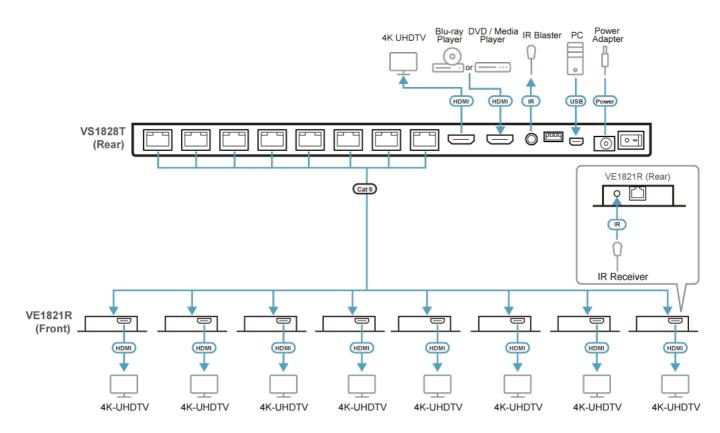
Note: Only connect VS1828T with VE1821R. Connecting VS1828T with other receiver models or third-party receivers may cause physical damage to the receiver.
