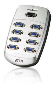
The VS88 Video Splitter duplicates the video signal from an input source (i.e. a computer) and route it to up to 8 display devices (monitors, projectors, etc.). However, they go beyond being merely duplicators, in that they also enhance the video signals over distances up to 30 meters. Furthermore, they can be cascaded three levels to additional ATEN video splitters to support many numerous display devices. And they mount inconspicuously on the wall or out of sight.
