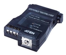
IC485AI is a 2-way converter converting RS-232 signals into RS-422/RS-485 signals in long-distance application up to 1200m (4000 ft.). Its built-in RS-485 automatic flow and direction monitoring function can suppress signal surge.
