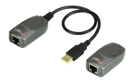
UCE260 can easily send the USB signals via Cat.5/5e/6 cable up to 60 meters (196 ft) at data rate of High Speed (480Mb/s) , Full Speed (12Mb/s) and Low Speed (1.5Mb/s). Without any configuration or software driver, this USB extender allows you to extend your USB device or hub up to 60m from your computer, which overcomes the typical USB cable limitation.
