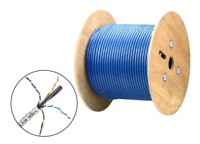
The 2L-2910 is a twisted pair cable engineered for optimum signal transmission at resolutions up to 4K including digital and analogue data, audio, and video applications. The cable supports sweep frequency up to 400 MHz and has been verified to meet performance requirements set by the HDBaseT Alliance.
