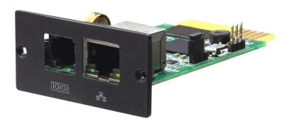
ATEN's SP100 (SNMP card) is an UPS monitoring equipment. Allows connection of the UPS directly to the ethernet network through a RJ-45 connector without using RS-232 ports on the computer and without loading any individual UPS management software on the network server. User can remotely control the UPS and monitor UPS current status from any off site location. SP100 can communicate the status of a UPS and issue commands to it.
