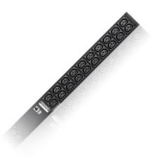
The PE2340 Energy PDU contains 40 AC outlets and is available in IEC or NEMA socket configurations. The PE2340 Energy PDU features a spacesaving 0U design that allows it to be mounted vertically on the outside of a rack, resulting in a more efficient use of space in the server room, while providing 40 AC outlets.
