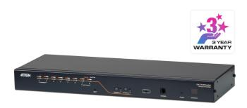
The KH2508A KVM switch is a control unit that allows IT administrators to access and control multiple computers from two PS/2 or USB KVM consoles (two bus). Operators working at up to two consoles can independently and simultaneously take control of up to 8 computers. By daisy chaining up to 31 additional switches, as many as 256 computers can be controlled from the original KVM consoles
