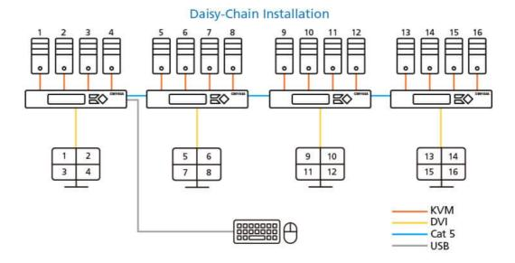
Furthermore, it can also be cascaded up to 2 levels by connecting additional 4 CM1164A units (up to 16 video sources) via a single console with video displayed in up to 4x4 multi-view mode.
