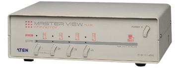
CS114A is a KVM Switch with built-in PS/2. It can control 4 servers via a single console and allows users to switch between computers via the buttons on the front panel of the switch or the hotkey configuration on the keyboard. It is the simplest and most convenient most convenient solution for multi-computer management.
