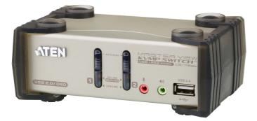
The CS1732B is 2-port KVM switch combined with a 2-port USB 2.0 hub. As a KVM switch, it allows users to access two computers from a single keyboard, monitor, and mouse console. There are four methods to obtain instant access to any computer in your installation: Pushbuttons, Hotkeys, OSD, and mouse.
