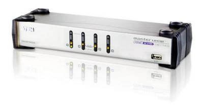
CS1744 KVM Switch integrates functions of video signal dual output and USB KVM switches. It allows a computer with dual-screen support to pair with two VGA/SVGA/Multisync displays via a USB keyboard and mouse. Furthermore, CS1744 provides 1 USB port on each of the front and rear panels, allowing each server to share any USB peripheral device that is connected to this HUB.
