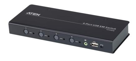
The CS724KM is a 4-Port USB KM Switch that enables users to control up to 4 computers with a single keyboard and mouse. Two switches can be daisy-chained to enable control of up to 8 computers from a single console.
