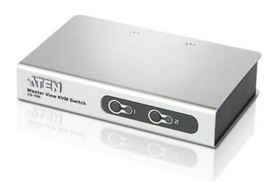
The KVM (Keyboard, Video, Mouse) switch is a control unit that allows access to two computers from a single console (keyboard, monitor, and mouse). With its custom designed connectors, the significantly reduces the number of ports required for a 2 port KVM switch. The design features a custom SPHD-15 male connector for the keyboard, video, and mouse, and SPHD-15 female connectors for the cables that connect the switch to the computers.
